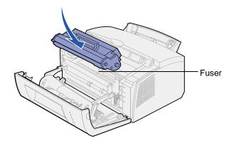
**c** Push down on the cartridge until it is firmly in place.
