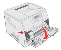
**2** Push the release latch, and open the top front cover.
