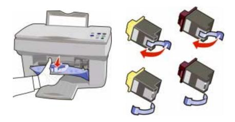
11 Place the cartridges into the carrier. Push back on the cartridges until they **snap** into place.
