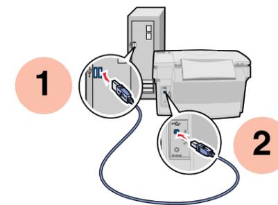
**Important:** If installation does not continue after connecting the USB cable, disconnect, and then reconnect both the USB cable and the power supply.
