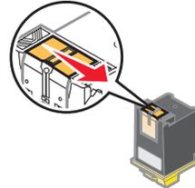
**Warning:** Wipe the nozzles in one direction so the colors do not mix.
