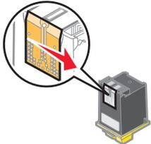
**Warning:** Do not wipe the nozzles and contacts with the same section of cloth.
