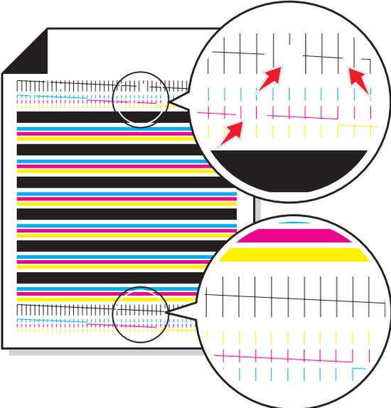
Compare the diagonal lines **above** the printed bars to the diagonal lines **below** the printed bars. Look for a break in the diagonal lines **above** the printed bars. Broken lines indicate clogged nozzles. Look for continuity in the diagonal lines below the printed bars. Unbroken lines indicate clean nozzles.
