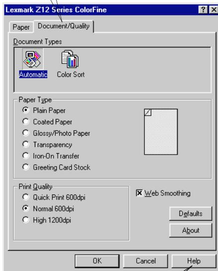
Click the **Help** button on either tab in the Printer Properties to access the printer driver Help.
