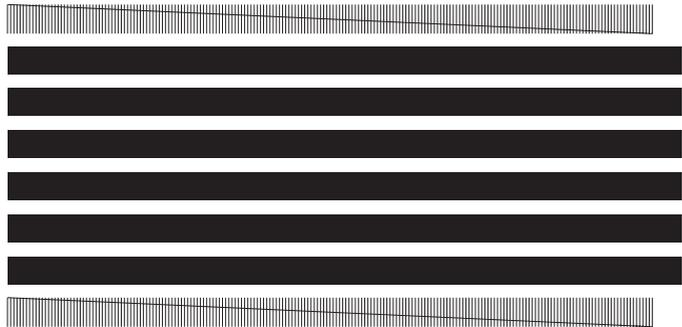
If you have a color cartridge installed in your printer, the printer prints a nozzle test pattern similar to the one shown:
