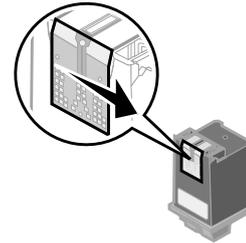
**b** Use another clean section of cloth to gently wipe the contacts. Hold the damp, lint-free cloth against the contacts for about three seconds. Gently blot and wipe dry.
