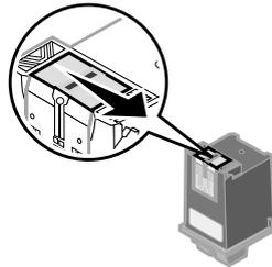
**a** Hold the damp cloth against the nozzles for about three seconds. Gently blot and wipe dry.
