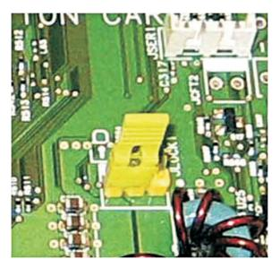
The secure reset feature requires specifying in the Embedded Web Server the effect of using the *security reset jumper*, which is located on the controller board.
