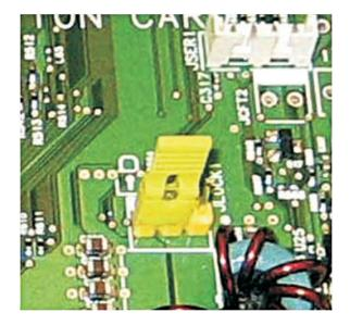
The secure reset feature requires specifying in the Embedded Web Server the effect of using the security reset *jumper*, which is on the controller board.
