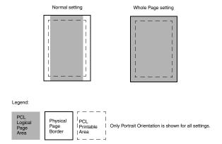
The printer holds this formatted image in memory. When the page prints, the image is compressed horizontally and vertically. The image is then centered on the physical page for letter size paper only. This process creates a small margin around the image. This artificial margin prevents printing from one edge to the other. Edge-to-edge printing could contaminate the printer and cause printing problems.
