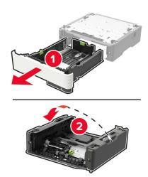
Remove the used pick roller assembly.
