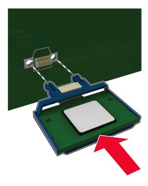
**Note:** The entire length of the connector on the card must touch and be flush against the controller board.
