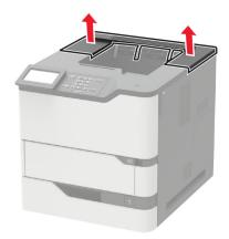
**6** Install the output expander on the printer, and then push it down to make sure that it is securely attached to the printer.
