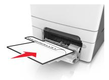
• Load envelopes with the flap side up and against the right side of the paper guide.
