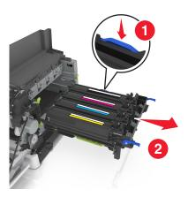
**8** Remove the used developer unit.
