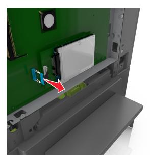
**3** Remove the printer hard disk by pulling it away from the controller board.
