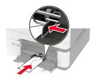
**Warning—Potential Damage:** Do not use envelopes with stamps, clasps, snaps, windows, coated linings, or self-stick adhesives.
