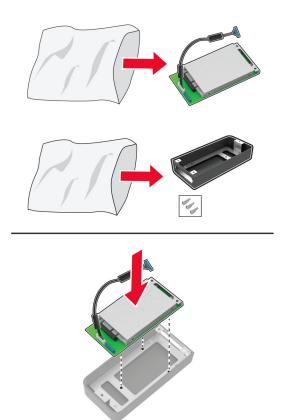
6 Attach the hard disk to the controller board access cover.
