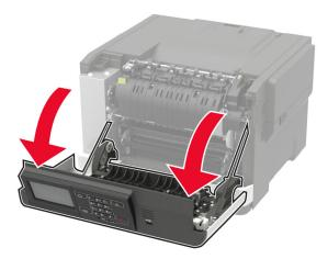
2 Open the fuser access door, and then remove the jammed paper.Note: Make sure that all paper fragments are removed.
