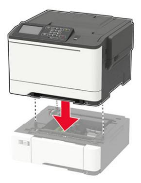
**Note:** If you are installing both the optional trays, then place the 550-sheet tray below the 650-sheet duo tray.
