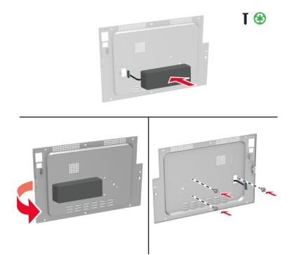
7 Connect the hard disk interface cable to the controller board, and then attach the access cover.
