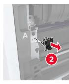
**4** Loosen the screws that secure the transfer belt.
