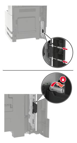
Connect the wireless print server to the controller board.
