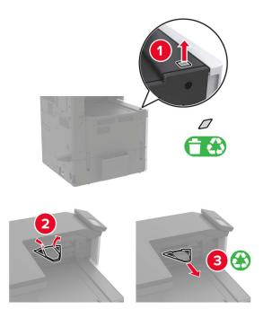
**6** Using the screwdriver stored inside door A, remove the covers for the paper guide sensor and slide rail.
