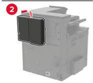
**5** Remove the controller board access cover.
