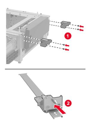
**13** Attach the rail, and then attach the mounting bracket and rail covers.
