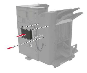
**16** Connect the power cord to the printer, and then to the electrical outlet.
