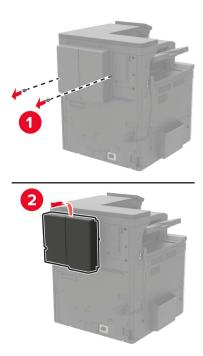
**5** Remove the controller board access cover.
