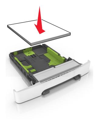
Make sure that the paper guides are positioned correctly and are not pressing tightly against the paper or envelopes.
