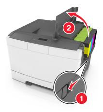
2 Remove the toner cartridge by lifting the handle, and then gently pulling it away from the imaging kit.
