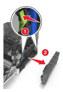
Lift the blue levers on the imaging kit, and then pull the imaging kit until it stops.
