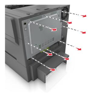
**3** Slightly open the controller board access cover, and then shift to the right to remove it.
