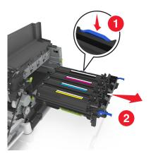
**8** Remove the used developer unit.
