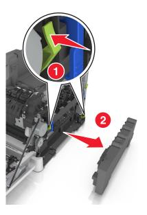
**6** Lift the blue levers on the imaging kit, and then pull the imaging kit until it stops.
