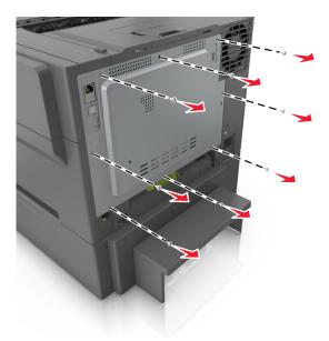
2 Slightly open the controller board access cover, and then shift to the right to remove it.
