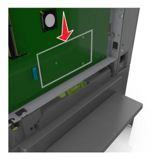
**5** Align the standoffs of the printer hard disk to the holes in the controller board, and then press the printer hard disk down until the standoffs are in place.
