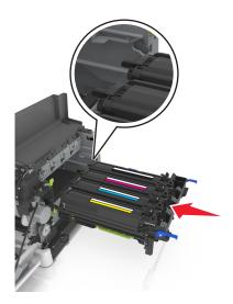
Push the blue levers down until the imaging kit is fully seated into place.
