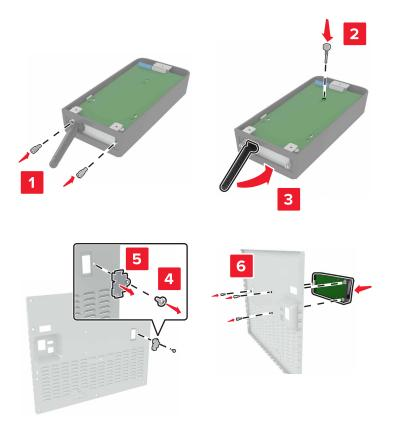
**6** Connect the ISP extended cable to the ISP connector in the controller board.
