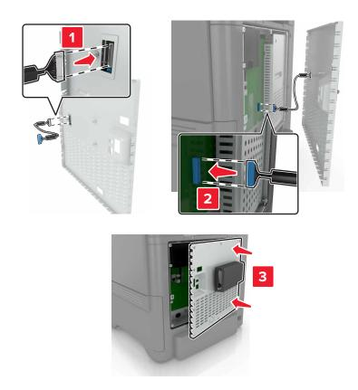
7 Reattach the controller board access cover.
