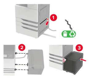
Attach the stabilizing feet to the printer.
