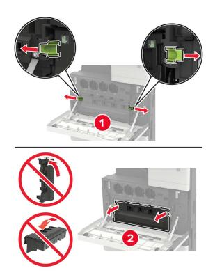
**3** Using the printhead wiper, clean the printhead lens.
