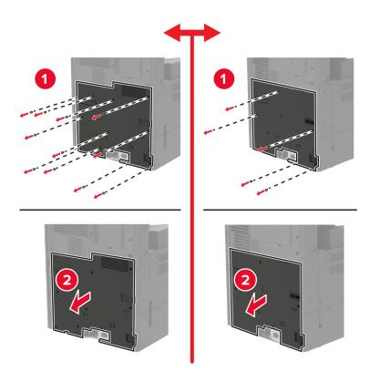
**6** Remove the controller board shield.
