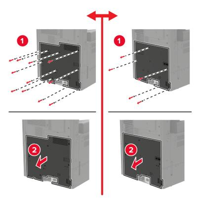
Remove the controller board shield.
