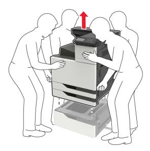
Remove the stabilizing feet from the tray.
