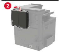
**5** Remove the controller board access cover.
