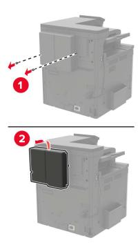
**5** Remove the controller board access cover.
