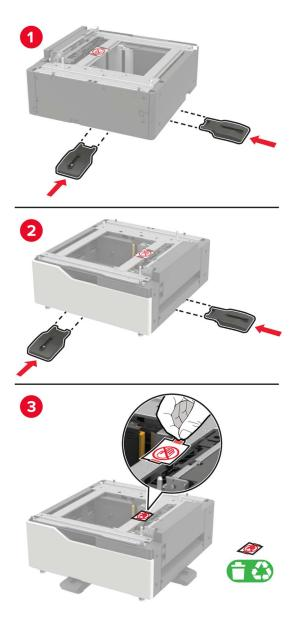
**5** Using the side handles, align the printer with the tray, and then lower the printer into place.
