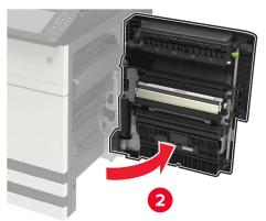
Using the screwdriver stored inside door A, remove the door stopper.
