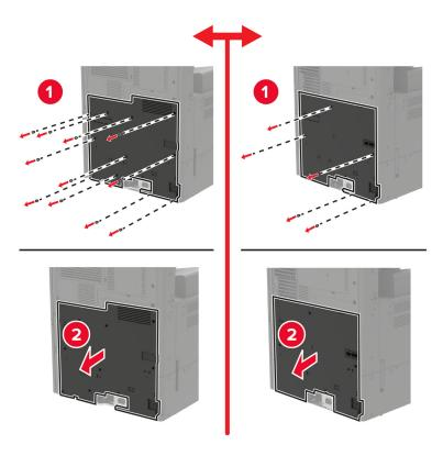
**6** Remove the controller board shield.
