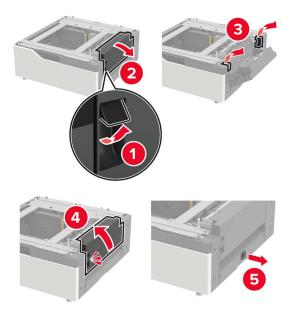
Open the tray, and then remove the mounting bracket and rail covers.
