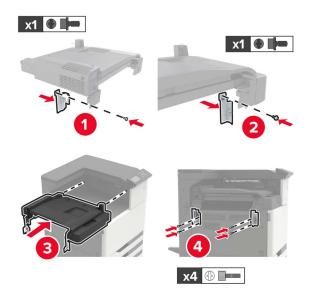
Attach the finisher to the printer.
