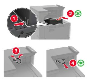
Using the screwdriver stored inside door A, remove the paper guides.
