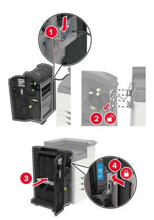
**9** Insert the staple cartridge into the finisher until it *clicks* into place.
