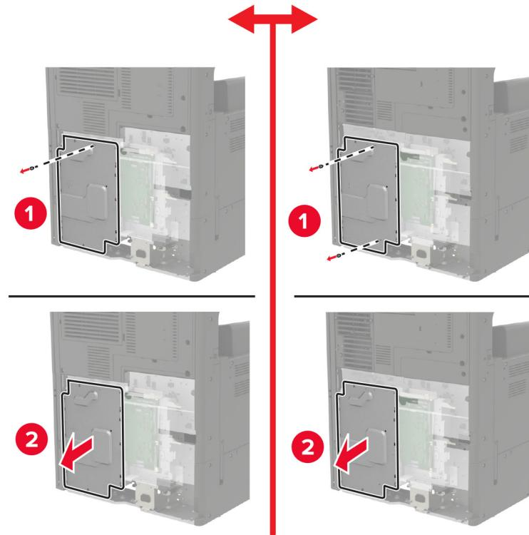
**5 打开端口通道盖门。**
