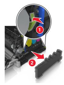
**6** Seal the used waste toner bottle in the enclosed packaging. For more information, see <u>"Recycling Lexmark products" on page 127</u>. 7 Insert the replacement waste toner bottle.
