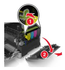
**5** Press the green levers on each side of the waste toner bottle, and then remove the waste toner bottle.
