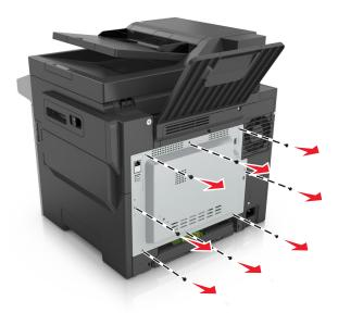
3 Slightly open the controller board access cover, and then shift to the right to remove it.
