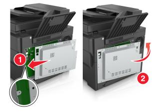
6 Turn the screws clockwise to lock the cover.
