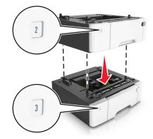
**4** Align the printer with the 650-sheet duo tray, and then lower the printer into place.
