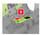
**4** Remove the ADF separator roller.
