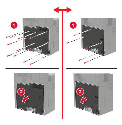
Remove the controller board shield.
