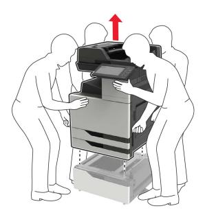
Remove the stabilizing feet from the tray.
