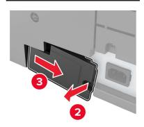
**4** If the printer has a filter cover, then remove the cover.
