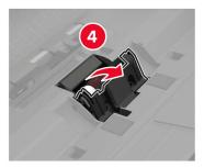
Remove the ADF separator roller.
