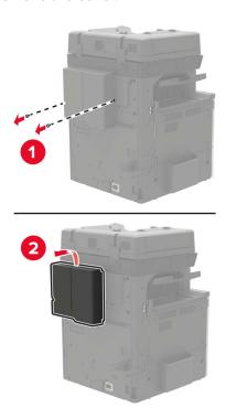
**5** Remove the controller board access cover.
