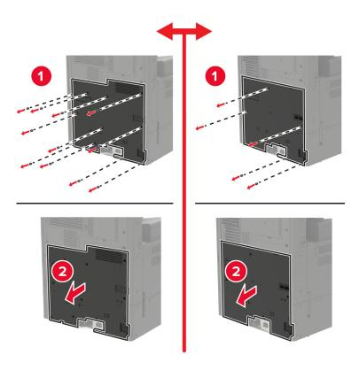
Remove the controller board shield.
