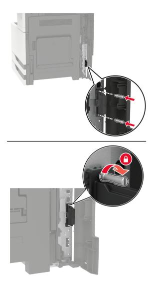
Connect the wireless print server to the controller board.
