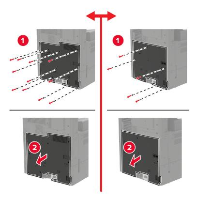
Remove the controller board shield.
