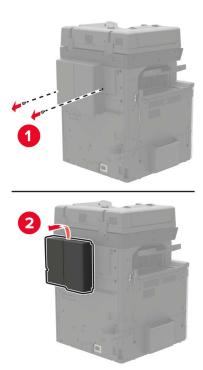
**5** Remove the controller board access cover.
