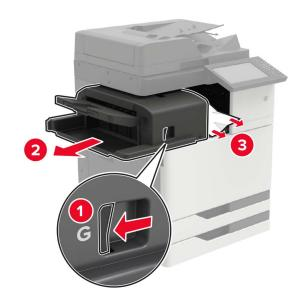
If necessary, turn the spinner wheel G1 downward to feed the jammed paper into the finisher bin, and then remove the jammed paper.
