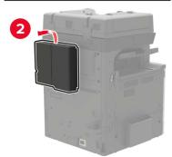
**5** Remove the controller board access cover.
