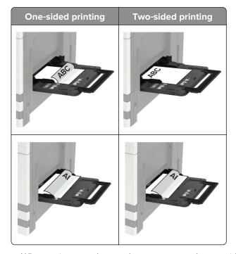
**Warning—Potential Damage:** When using envelopes, do not use envelopes with stamps, clasps, snaps, windows, coated linings, or self-stick adhesives.
