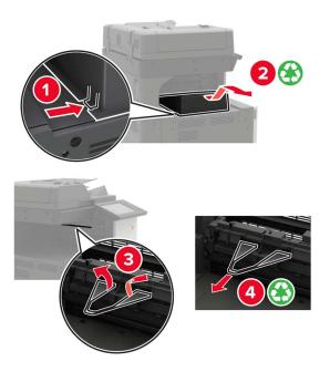
Using the screwdriver stored inside door A, remove the paper guides.
