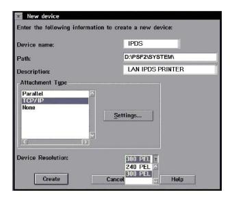
Enter the device name and the device description and select a Device Resolution of 300 pel.
