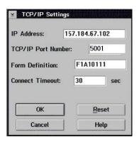
Enter the IP address of the printer. The IP address should be obtained from your network administrator. Enter the TCP/IP port selected in Step 1.
