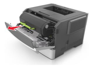
Lift the green handle, and then pull the imaging unit out of the printer.
