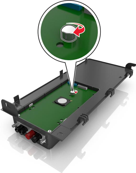
7 Tighten the two screws on the end of the ISP solution.
