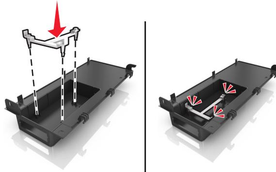
**5** Slide and push the ISP solution into the plastic bracket.
