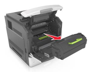
**3** Lift the green handle, and then pull out the imaging unit from the printer.
