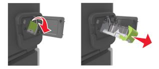
**3** Squeeze both sides of the empty staple case with your fingers, and then remove the staple case from the cartridge.
