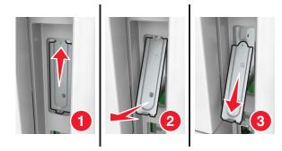
**5** Align the posts of the plastic bracket with the holes on the controller board cage, and then press the plastic bracket on the controller board cage until it *clicks* into place. Make sure the cables are neatly tucked under the plastic bracket.
