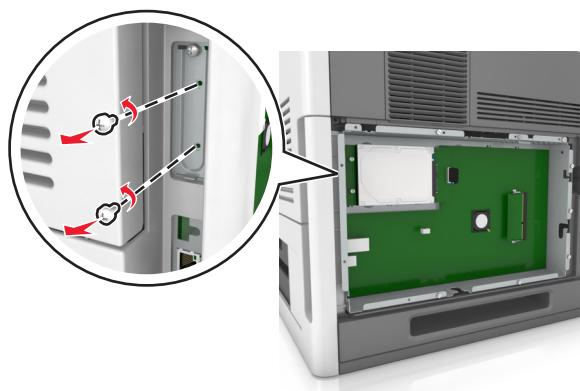
**4 移除打印机硬盘。**
