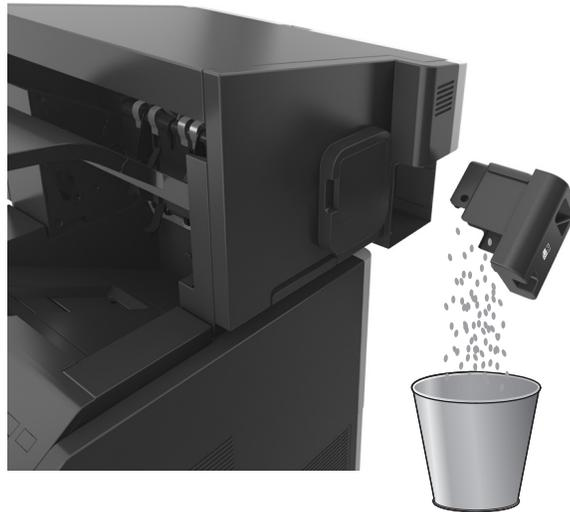
**3** Insert the emptied hole punch box back into the finisher until it *clicks* into place.
