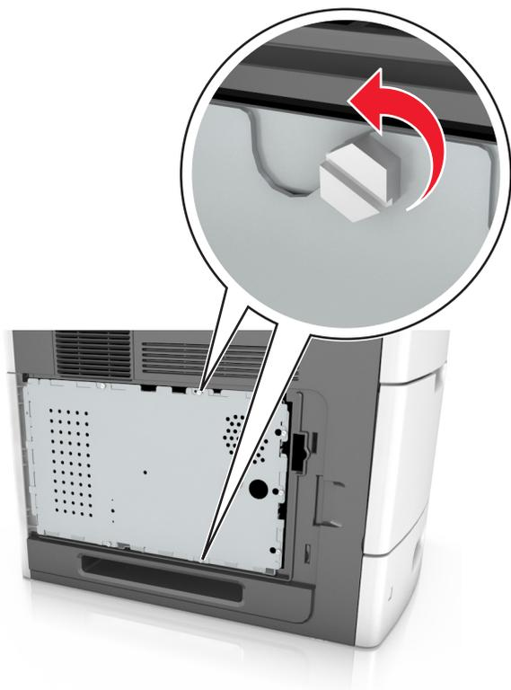
**3** Remove the shield.
