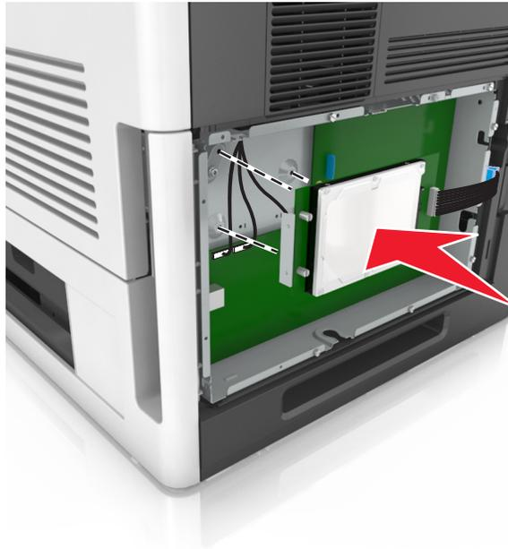
**Note:** Make sure the cables are neatly tucked under the printer hard disk.
