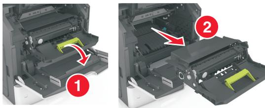
**Warning—Potential Damage:** Do not expose the imaging unit to direct light for more than 10 minutes. Extended exposure to light may cause print quality problems.
