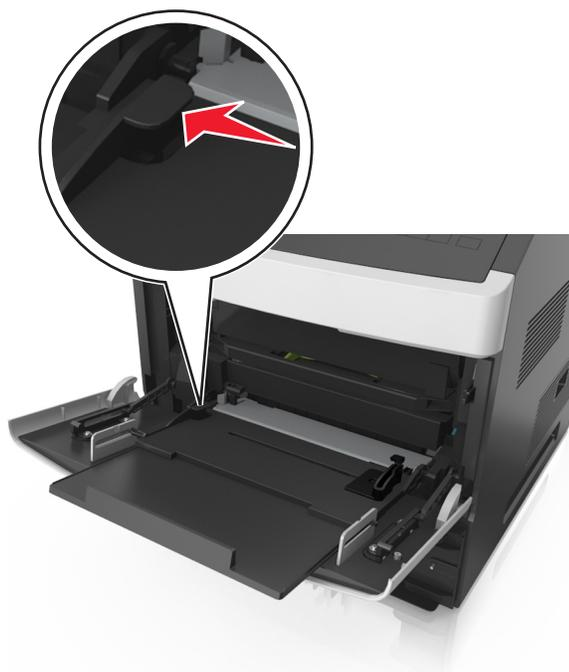
**Warning—Potential Damage:** Overfilling the feeder can cause paper jams.
