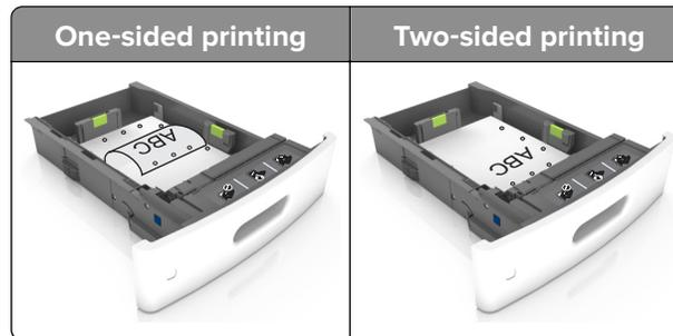
**Note:** If the holes on the long edge of the paper are on the left side of the tray, then a jam may occur.
