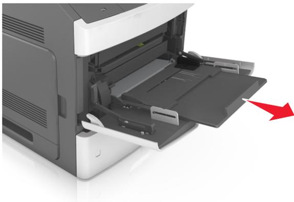
**Note:** Guide the extender gently so that the multipurpose feeder is fully extended and open.
