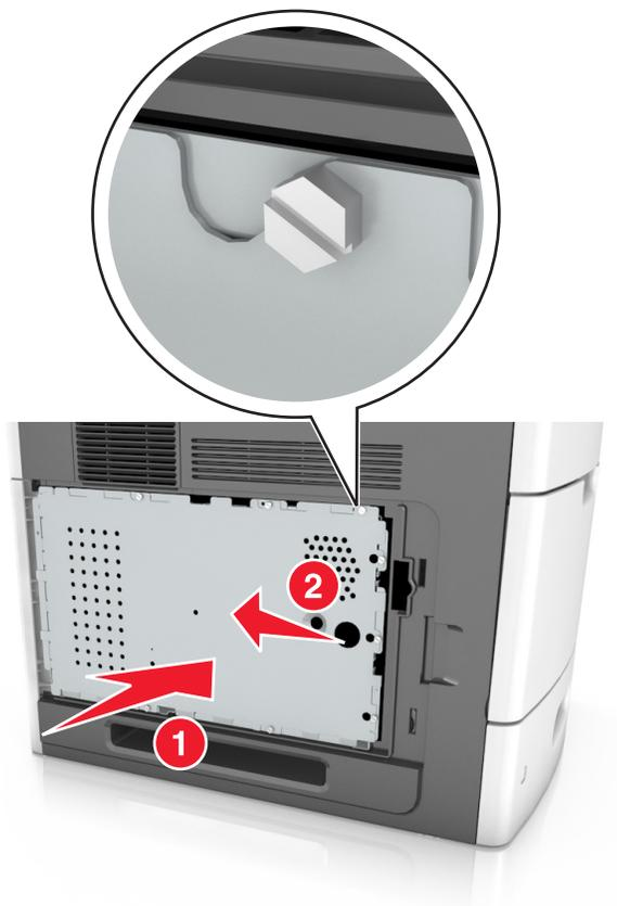
6 Tighten the screws on the shield.
