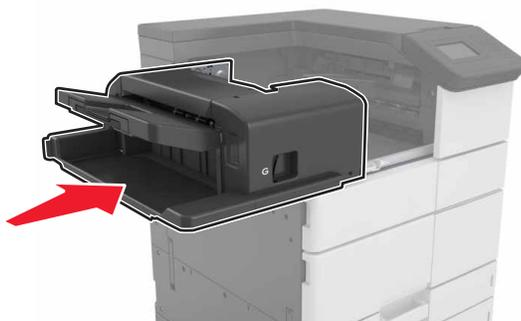
**[x]-page jam, open door H and rotate knob H6 clockwise.
