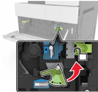
4 Remove the photoconductor unit.
