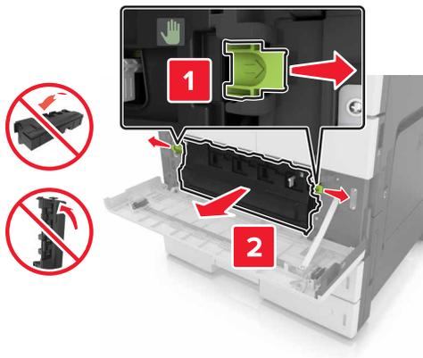
3 Unlock the photoconductor unit.
