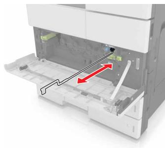
**5** Remove the printhead wiper.
