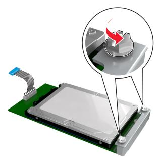
b Insert the plug of the printer hard disk interface cable into the receptacle of the controller board.Note: The plug and the receptacle are color-coded blue.
