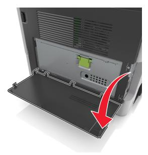
2 Lightly press the stop on the left side of the access door, and then slide the access door to remove it.
