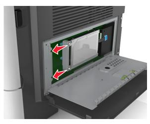
**d** Tighten the two screws.
