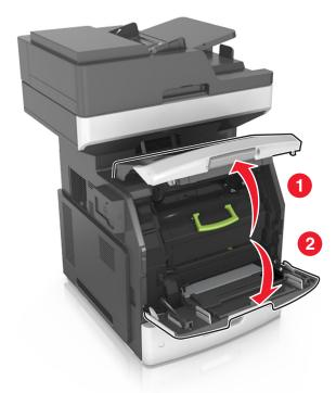
**2** Pull the cartridge out of the printer using the handle.
