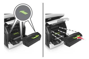
**Warning—Potential Damage:** When replacing a toner cartridge, do not leave the imaging unit exposed to direct light for an extended period of time. Extended exposure to light may cause print quality problems.
