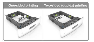
• Do not slide the paper into the tray. Load paper as shown in the illustration.
