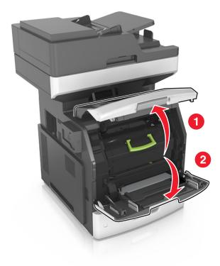
**2** Pull out the toner cartridge from the printer using the handle.
