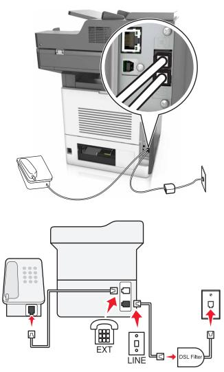
Digital subscriber line (DSL) splits your regular telephone line into two channels: voice and Internet. Telephone and fax signals travel through the voice channel, and Internet signals pass through the other channel.
