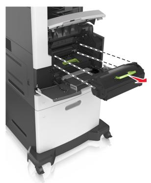
${\bf 3}~$  Lift the green handle, and then pull out the imaging unit from the printer.
