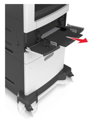
Note: Guide the extender gently so that the multipurpose feeder is fully extended and open.
