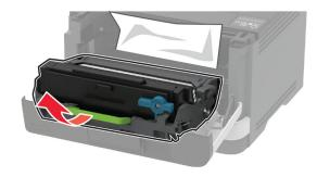
**Warning—Potential Damage:** Do not expose the imaging unit to direct light for more than 10 minutes. Extended exposure to light may cause print quality problems.
