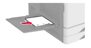
• For two-sided printing, load letterhead faceup with the header to the left side of the paper. Load hole-punched paper faceup with the holes toward the front of the printer.
