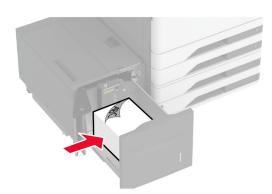
• Load prepunched paper facedown with the holes against the left side of the tray.
