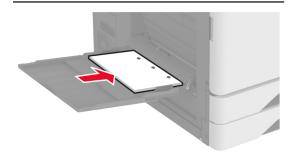
• For two-sided printing, load letterhead faceup with the header toward the rear of the printer. Load hole-punched paper faceup with the holes to the left side of the paper.
