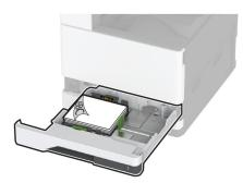
• Load prepunched paper facedown with the holes against the back of the tray.
