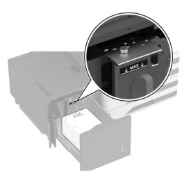
6 Close the tray side door, and then insert the tray.If necessary, set the paper size and type to match the paper loaded in the tray.
