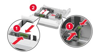
**4** Load the envelopes with the flap side down and against the left side of the tray.
