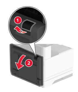
9 Open door C, and then remove the jammed paper.
