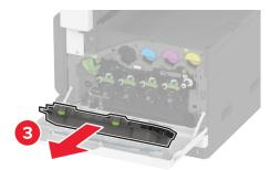
**Note:** To avoid spilling the toner, place the bottle in an upright position.
