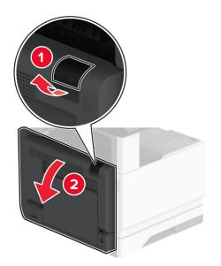
2 Open door A1, and then remove the jammed paper.Note: Make sure that all paper fragments are removed.
