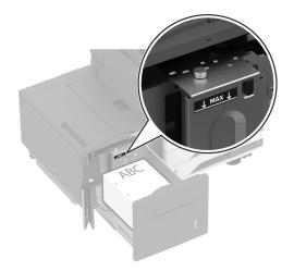
6 Close the tray side door, and then insert the tray.If necessary, set the paper size and type to match the paper loaded in the tray.
