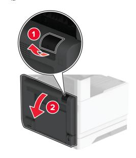
**2** Open door A1, and then remove the jammed paper. Note: Make sure that all paper fragments are removed.
