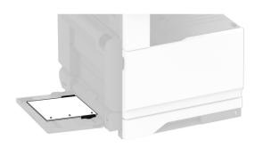
For two-sided printing, load letterhead faceup with the header to the left side of the paper. Load hole-punched paper faceup with the holes toward the front of the printer.
