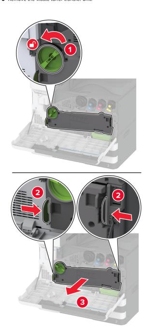
**Note:** To avoid spilling the toner, place the unit in an upright position.
