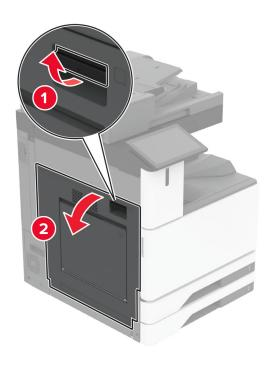
**2** Open door C, and then remove the jammed paper.
