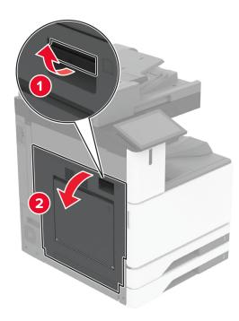
**9** Open door C, and then remove the jammed paper.
