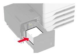
**Note:** Make sure that the stack height is below the maximum paper fill indicator. Overfilling may cause paper jams.
