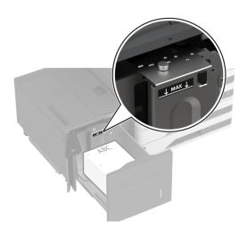
**6** Close the tray side door, and then insert the tray. If necessary, set the paper size and type to match the paper loaded in the tray.
