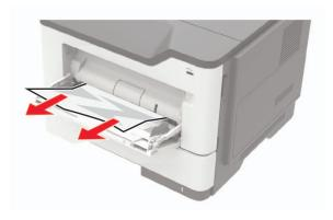
Flex, fan, and align the paper edges before loading.
