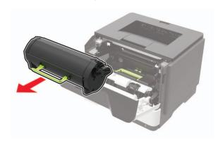
**3** Remove the used imaging unit.
