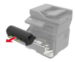
**3** Remove the used imaging unit.
