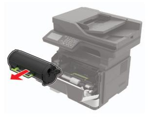
**3** Remove the used imaging unit.
