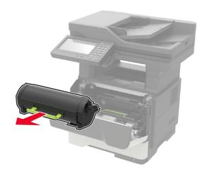
**3** Remove the used imaging unit.
