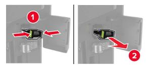
Lift the staple guard, and then remove the loose staples.
