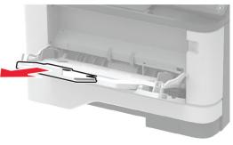
**10** Flex, fan, and align the paper edges before loading.
