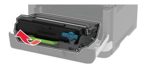
**Warning—Potential Damage:** Do not expose the imaging unit to direct light for more than 10 minutes. Extended exposure to light may cause print quality problems.
