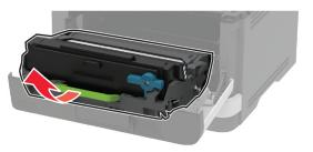
**3** Twist the blue latch, and then remove the used toner cartridge from the imaging unit.
