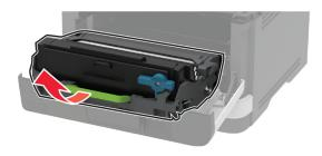
Twist the blue latch, and then remove the used toner cartridge from the imaging unit.
