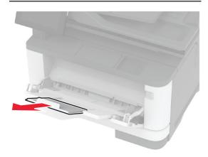
**10** Flex, fan, and align the paper edges before loading.
