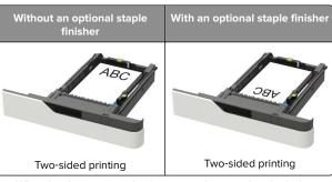
When loading prepunched paper, make sure that the holes on the long edge of the paper are against the right side of the tray.
