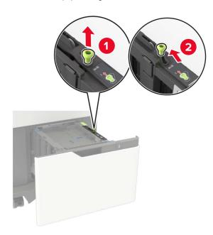
b If the A5 length guide is still attached, then remove it. If the guide is not attached, then proceed to <a href="step d on page">step d on page</a>
