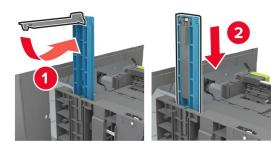
**d** Squeeze, and then slide the length guide to the correct position for the size of the paper being loaded.
