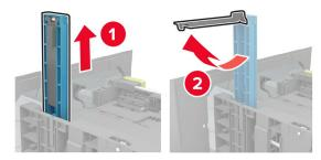
**d** Insert the guide into its designated slot, and then press until it *clicks* into place.
