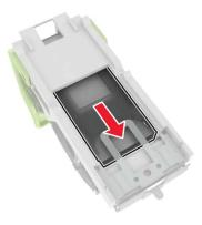
**Note:** If the staples are at the rear of the cartridge, then shake the cartridge downward to bring the staples near the metal bracket.
