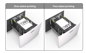
**Note:** If the holes on the long edge of the paper are on the left side of the tray, then a jam may occur.
