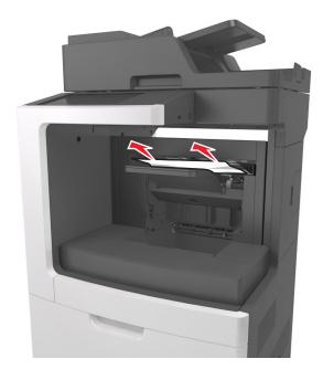
**2** Open the staple finisher rear door, and then remove the jammed paper.
