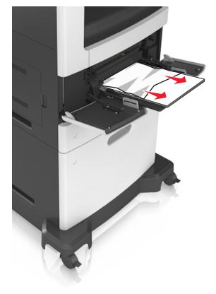
**3** Flex, fan, and align the paper edges before loading.
