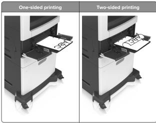
**Note:** If the holes on the long edge of the paper are on the left side of the tray, then a jam may occur.
