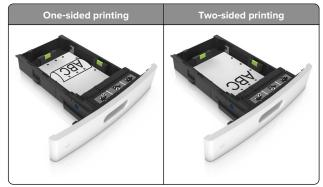
**Note:** If the holes on the long edge of the paper are on the left side of the tray, then a jam may occur.
