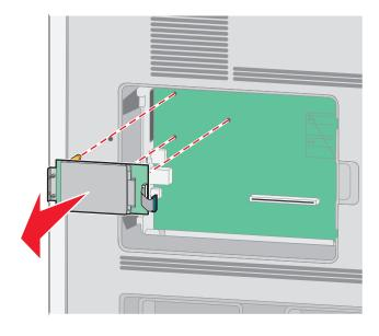
**d** Remove the thumbscrews that attach the printer hard disk mounting bracket to the printer hard disk, and then remove the bracket. Set the printer hard disk aside.
