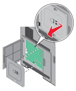
**4** Use the illustration below to locate the appropriate connector.
